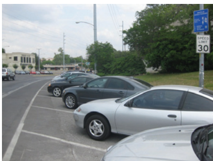
Back-in angle parking in Austin, TX with adjacent instructional sign (blue sign above speed limit sign)
