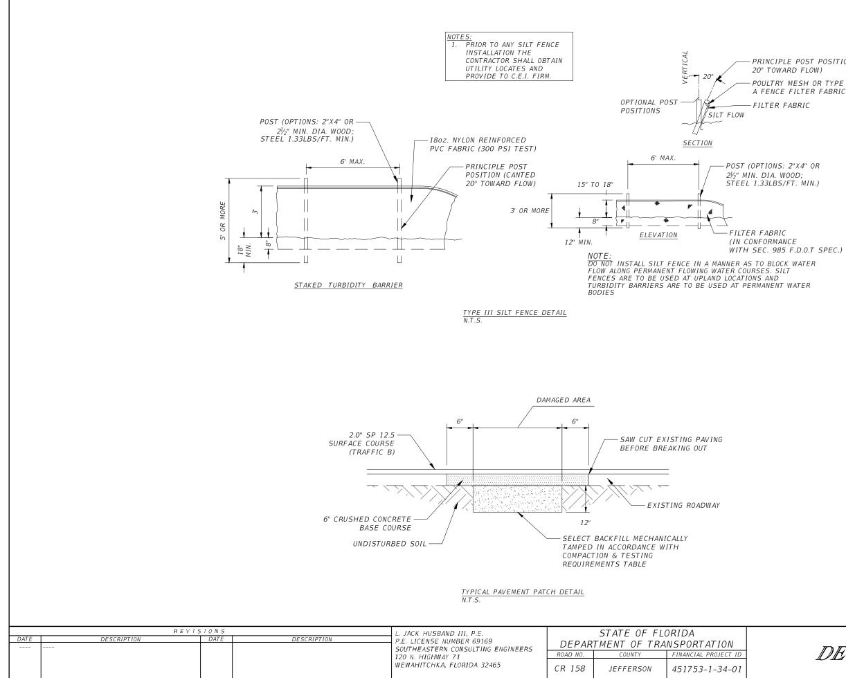
PRINCIPLE POST POSITION (CANTED POULTRY MESH OR TYPE A FENCE FILTER FABRIC
